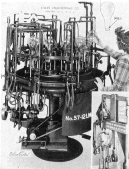
The Eisler automatic neck-molding and bulb sealing-in machine. (Patent No. 2,418,763.)
